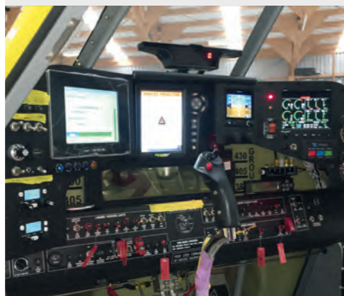
Avionics installations underway on an Air Tractor
