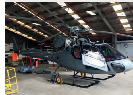
AS350 B2 maintenance underway
