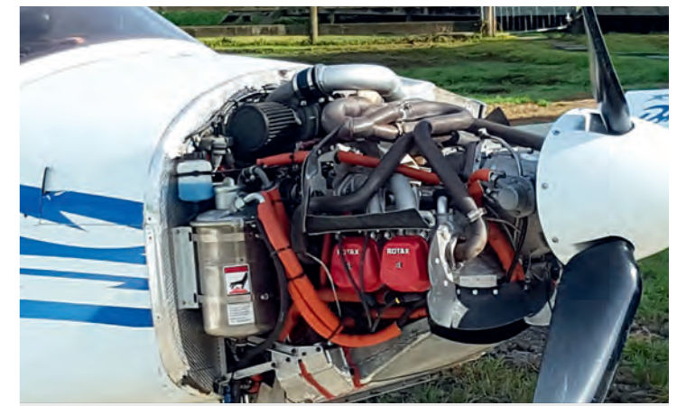
914 intercooled turbo DynAero installation - 160 kts at 10000 ft
